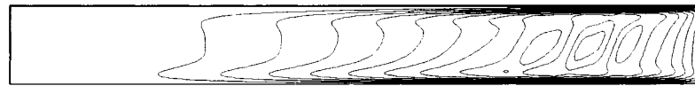
Fig. 2. Meridional streamline contours obtained with different grid systems for Ek = 0.0057 , Sc Ro_s = 10.63 , Ar = 0.033 (vertical scale 3 \times ).
